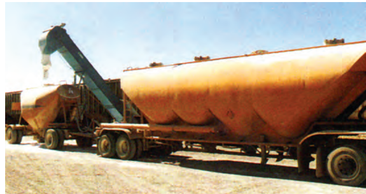
Pebble Lime: Unloading at 150 TPH
