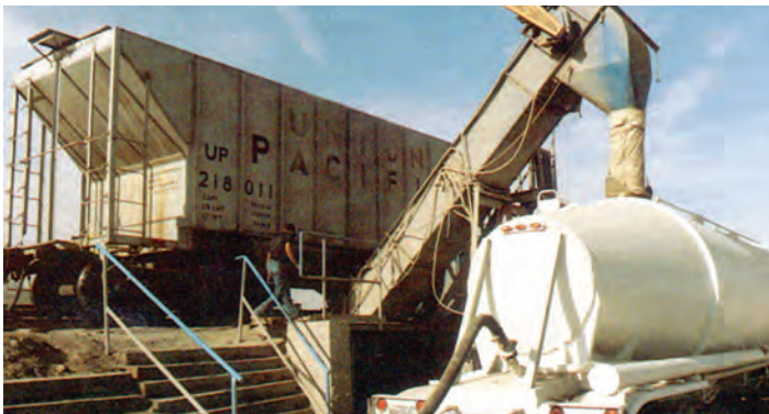
Cement: Unloading at 120 TPH
