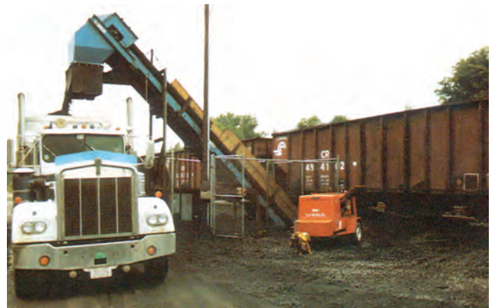
Coal: Loading 24 tons in 4 minutes (360 TPH).
