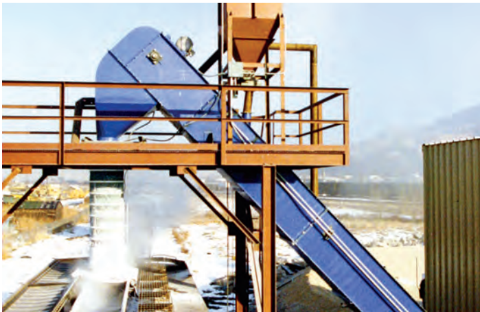
Soda Ash: Unloading 80,000 lbs. in 20 minutes (120 TPH).
